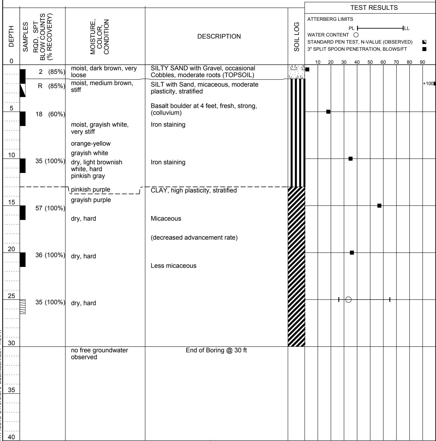
LOGS WITHOUT WELL WITH TESTS S17073.GPT BUDINGER GDT 7/31/17
