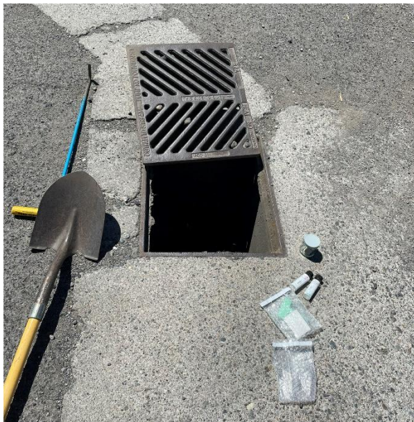
SAMPLES BEING TAKEN OF SEDIMENT IN A CATCH BASIN.
